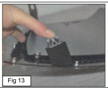
Put into place the (2)Brackets and using the (2)Flange Nuts, fix the Bracket to the new grille Replacement.
