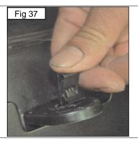
19 Remove all the fastener clips from the factory grille that was cut off from the shell. (Fig 38-39)
