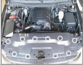
Open vehicles hood. Using a 10mm socket locate and remove 4 bolts circled above. Set hardware aside for re-installation.
