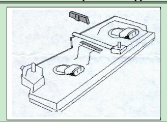
A portion of material must be cut from the core support to mount the headlamps. Use this diagram on the left to cut the area needed to recess the headlights. Make your cut as indicated by the shaded areas.
