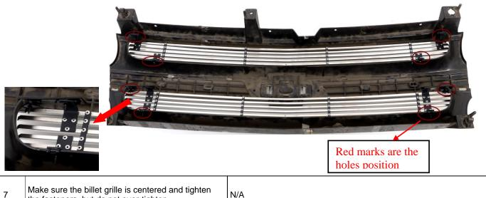
the fasteners. but do not over-tighten. Reinstall the black plastic cover which was removed 8 in step 2. Installation completed!!!
