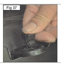
Remove all the fastener clips from the factory grille that was cut off from the shell. (Fig 38-39)
