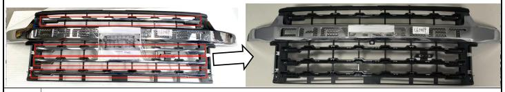
Thread a Stud in each nut welded to the grille. From the rear, place a Tab on each Stud. Now thread a Hex Flange Nut on each Stud.
