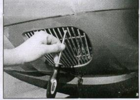
Figure 2 - Marking drill locations
