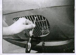
Figure 2 - Marking drill locations
