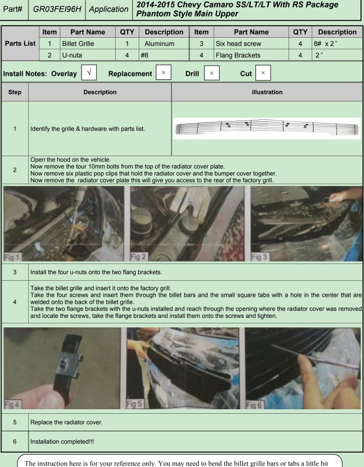
to adjust to fit. We strongly recommend the professional installer for best result. Please use masking tape and tape the OEM grille shell along the edge to protect your vehicle during installation.
