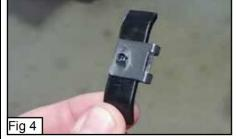
5.Install the two u-nuts onto the two flange brackets (Fig 4).
