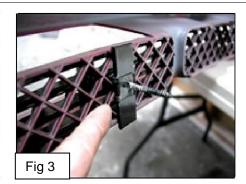
5 Make sure the billet grille is centered and tighten the fasteners, but do not over-tighten. 6 Reinstall the black plastic cover which was removed in step 2. 7 Installation completed!!!
