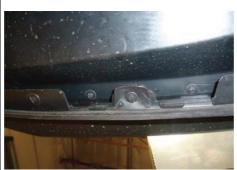
5. Remove 12 bolts on the inner bumper shell between the outer bolts.
