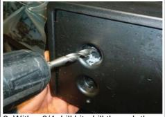
2. With a 3/4 drill bit, drill through the center of the screws on license plate and remove.
