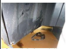
4. Remove 2 clips from each side fender well.
